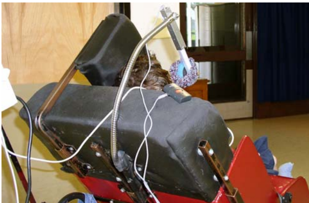
Adapted for a wheelchair, this electronic communications device issues prerecorded messages.
